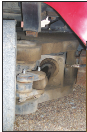
Steer cylinder is completely protected in axle housing.
